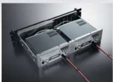
Two RF units can be installed inside. (Left side is an option.)
