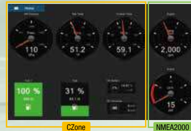
CZone, engine, navigation and various NMEA2000 data can be laid out on the same screen.
